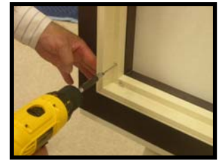
Only secure one screw into the bottom left frame.
